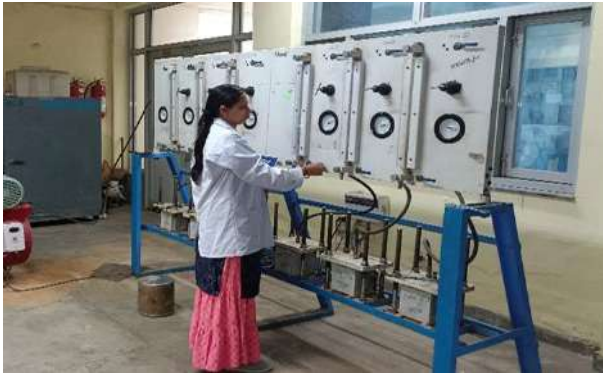
Water penetration testing for concrete
