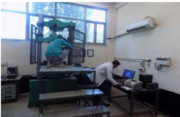
Universal testing machine- 1000kN for testing of reinforcement steel
