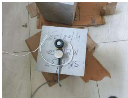
Fig: Evaluation of specific heat of concrete using TPS 500
