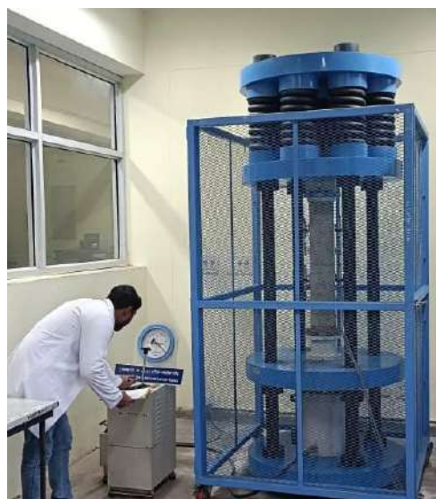
Hardened Concrete Sample CREEP Observation
