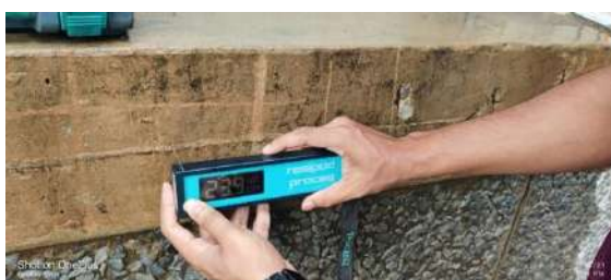
Measurement of surface electrical resistivity on an identified beam in NCB premises
