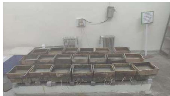
Concrete slab specimens selected for installation of anodes w.r.t Laboratory Study Under Chloride Induced Corrosion
