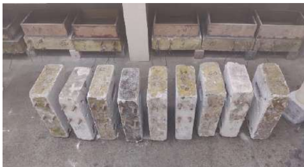
Concrete slab specimens selected for installation of anodes w.r.t Laboratory Study Under Carbonation Induced Corrosion
