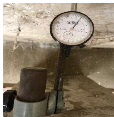
Determination of load carrying capacity by Load Testing of railway over bridge as per IRC SP-37 in progress at a sponsored project site
