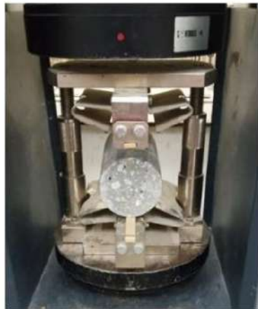
Test set-up for split tensile and flexural strength
