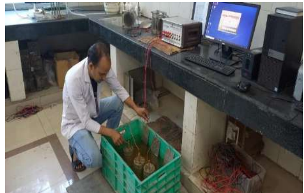
Accelerated corrosion testing (Florida method) of concrete
