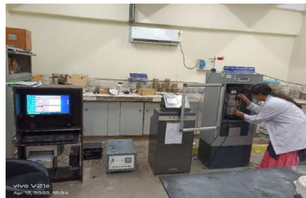
Strain Controlled Flexural Testing Machine for determination of flexural toughness of concrete
