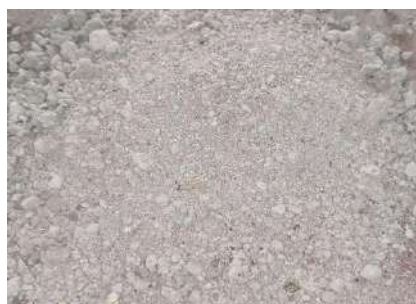
Fig: Processed LD slag as fine aggregate
