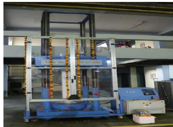
Column testing machine for checking behaviour of reinforced column
