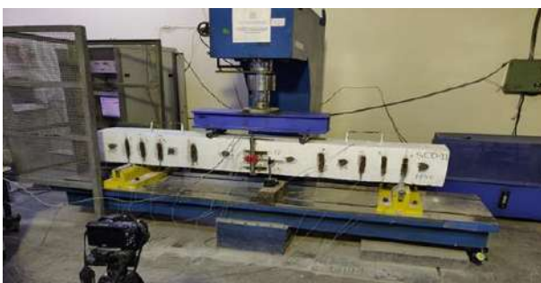
Flexural testing machine- 500kN for testing reinforced beam
