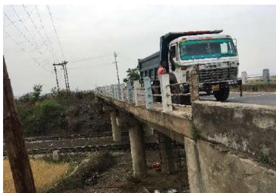
Determination of load carrying capacity by Load Testing of railway over bridge as per IRC SP-37 in progress at a sponsored project site
