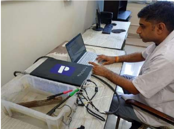
Corrosion Rate using Electrochemical Impedance Spectroscopy
