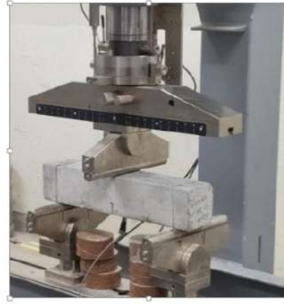
Test set-up for split tensile and flexural strength
