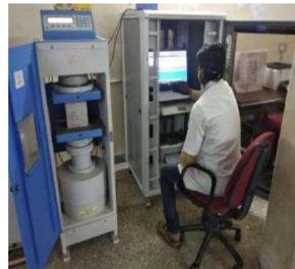
M35 Concrete Cubes Testing for Sponsored Projects
