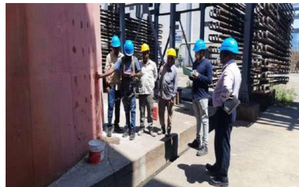
Half Cell Potential Test/ Strengthening Measures at NTPC Tanda
