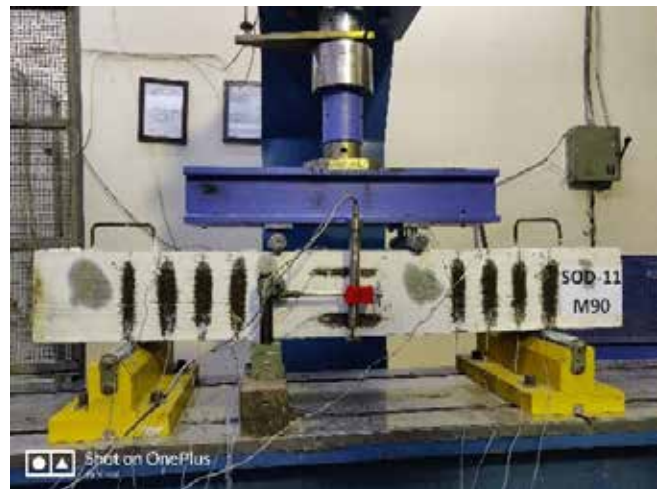
Figure-1 Test Set up for High Strength Concrete Reinforced Beams in Shear
