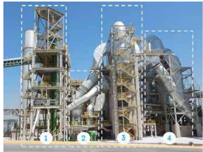
Fig-1: Standardized grinding plant module: quadropol® vertical roller mill
